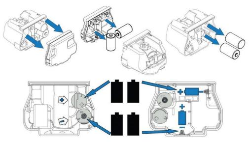
Once the batteries are inserted, replace the cover and refit the reservoir and pump mechanism back into the dispenser housing.
